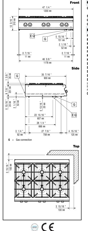
Modular Cooking Range Line EVO900 6-Burner Gas Boiling Top
